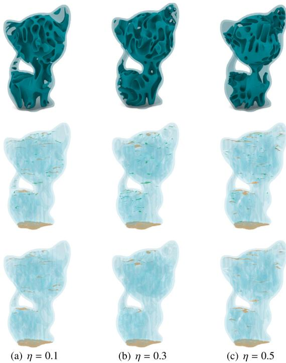
**Fig. 14.** Parameter setting in the small area filtering function. The top row is the optimized TPMS-based porous structures. The models in the middle row show the removable overhang regions and the actual overhang regions colored in green and orange, respectively. The bottom row shows the final overhang regions in the models. (For interpretation of the references to color in this figure legend, the reader is referred to the web version of this article.)
