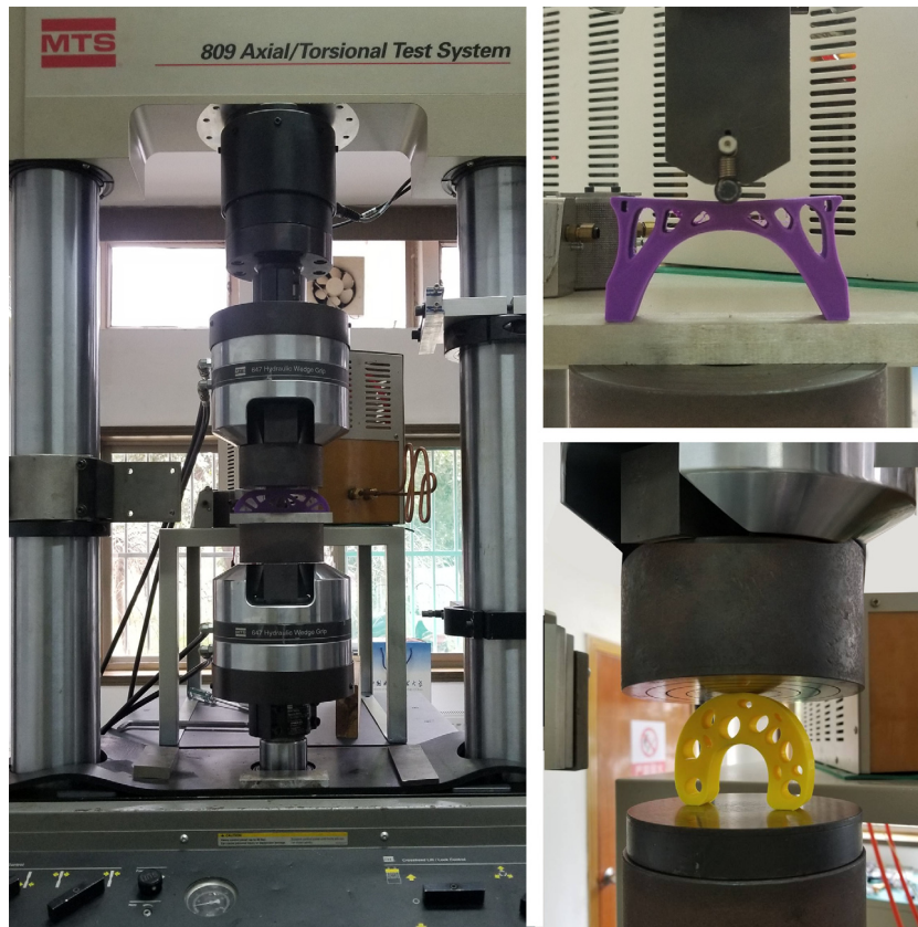
Fig. 14. Compression test using MTS809.
